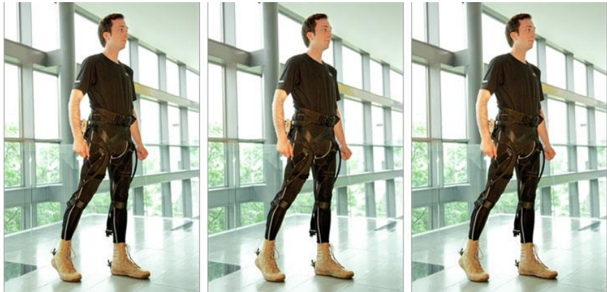
Harvard Exosuit: Rehabilitation / Injury Avoidance
